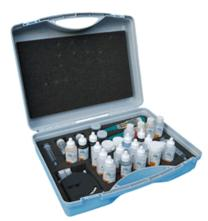
Boiler water and boiler feedwater systems require careful test monitoring to ensure the correct water conditions are maintained at all times. Failure to maintain the correct water treatment programs can lead to serious problems including reduced boiler efficiency, scale, corrosive water conditions and reduced steam purity.
